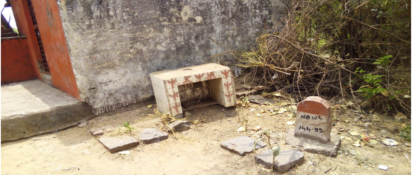
New Back Water Level marked as 144.92 M, in front of a temple in Ghazipura
